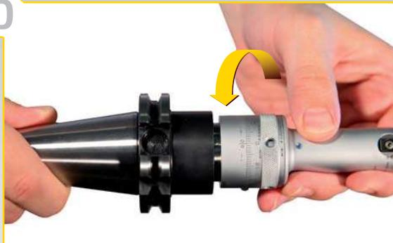
D. Screw the front end of the Taper Shank (2) onto the Differential Connector (5), now located at the back on the Boring Head (1). Screw carefully until the Positioning Pin (6) gently touches the Taper (2) face. Stop!
