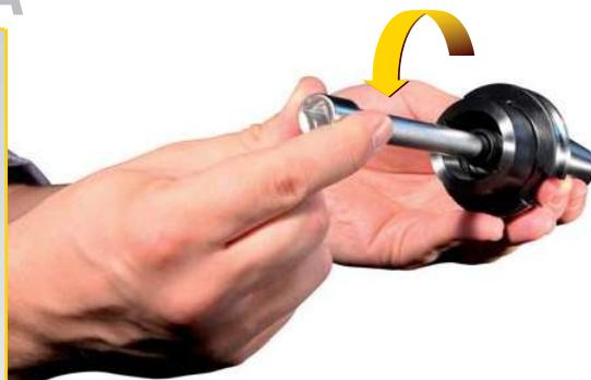
A. Remove the Differential Connector (5) from the Taper Shank (2).
