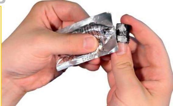
B. Lubricate the thread on the Differential Connector (5) with Lubricant ASL-3G (7), supplied with the Taper Shank (2).
