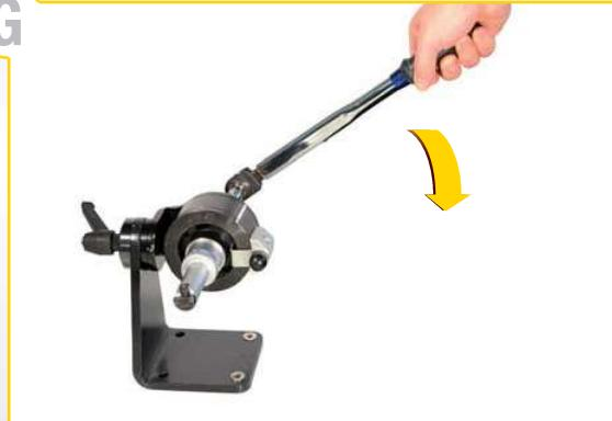
G. Tighten the Differential Connector (5) with the specified required torque, as shown on the table below. Use the Torque Wrench (4) to do this.
