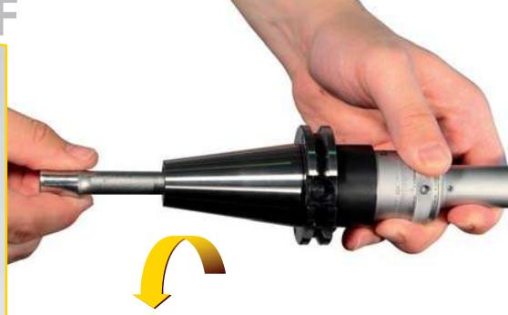
F. Insert the square end of the Extension (3) through the Taper Shank (2) and into the Differential Connector (5). Keeping the Positioning Pin (6) and the positioning slot aligned, turn the Extensions (3) anti-clockwise until you see that two Romicron faces are meshing. Ensure that the Positioning Pin (6) is inserted into the slot on the Taper Shank (2).
