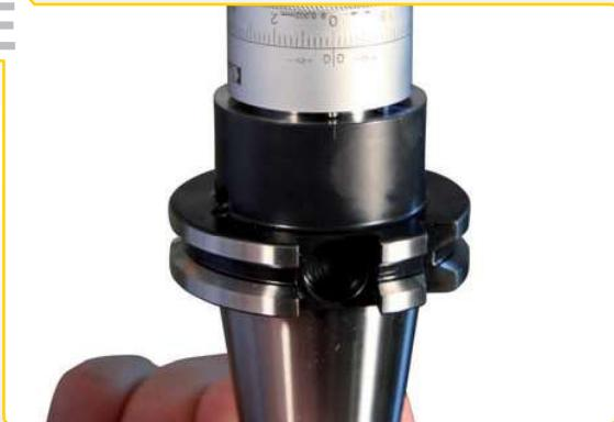
E. Unscrew the Taper Shank (2) a little bit until the Positioning Pin (6) is aligned with the positioning slot mark in the Taper Shank (2) face.
