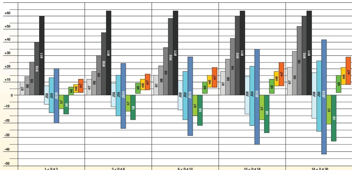
Achievable hole tolerance in  $\mu\text{m}$  per diameter range (mm).
