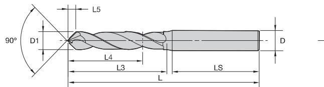
For information on L, L3, and L4 max, see the Solid Carbide Drills foldout table.
