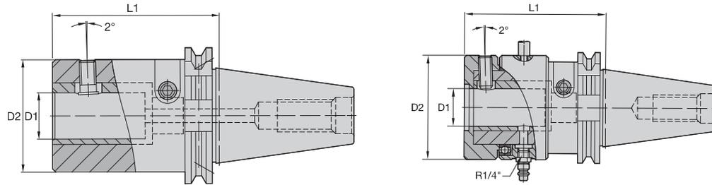
■ Drill Fix Chucks • Eccentric Adjustment Mechanism
