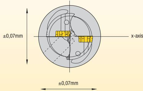
Metric shank drills with a 2° Whistle Notch shank are easily mounted into inch turrets using a WD adaptor. Align the X-axis of the drill with the X-axis of the machine tool as described above. Accurate alignment is absolutely essential for good performance. The drill must be on centre within the tolerance shown above. Angularity must not exceed 0,07mm.
