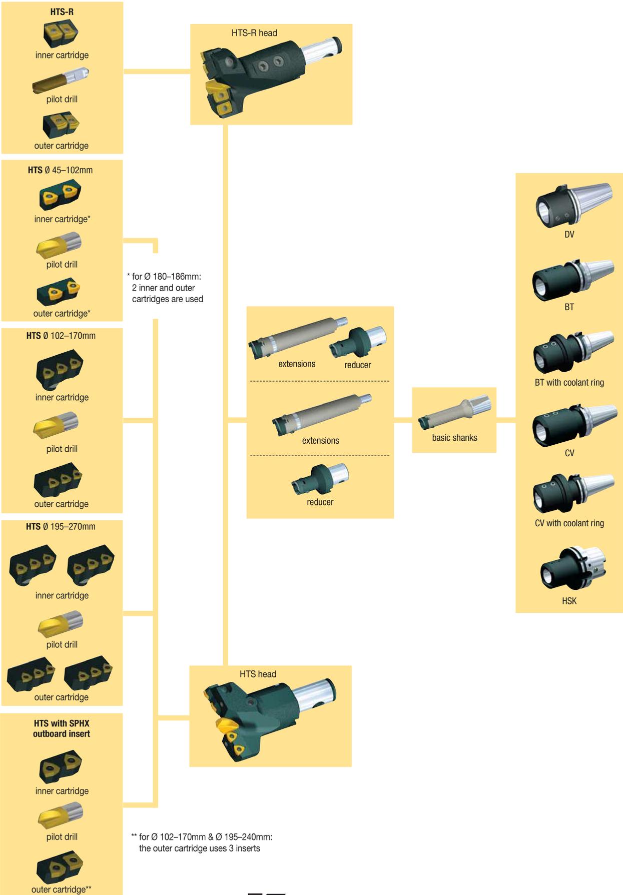
To assemble your HTS(-R) head, choose the desired drill diameter range from the left-hand column.
