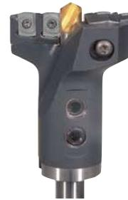
Install inner insert into cartridge.
