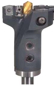
Install inner cartridge, then the outer insert.
