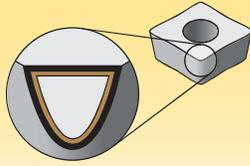
Coatings provide high-speed capability and are engineered for finishing to light roughing.
