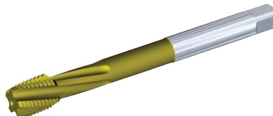
■ **T651 • Extra Long • Form C Semi-Bottoming Chamfer • Through Coolant • Larger Sizes • Metric • For Steel and Cast Iron**
